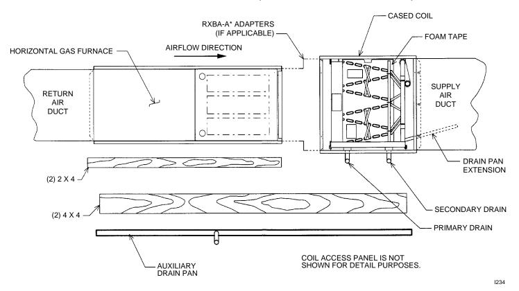
FIGURE 4. RIGHT-HAND AIR SUPPLY (FRONT CONNECTION COIL SHOWN)
