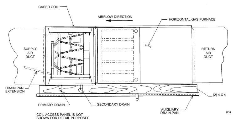
FIGURE 3. LEFT-HAND AIR SUPPLY (SIDE CONNECTION COIL SHOWN)
